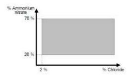
The shipper shall declare the ammonium nitrate content and the chloride content in accordance with 4.2 of this Code. Notwithstanding the above, fertilizers within these composition limits are not subject to the provisions of this schedule, if they are assigned class 9 due to the hazard of self-sustaining decomposition based on the results of the trough test (referred to in the UN Manual of Tests and Criteria, part III, section 39).
